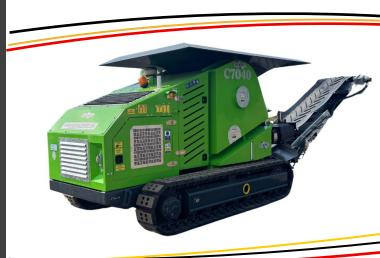
Crusher C7040 A 700 x400 Jaw crusher for processing a wide variety of materials including concrete, rubble and recycled hardcore. The material is fed directly into the jaw chamber. This hopper is lined with Hardox for long life. The crushed material is then discharged onto the conveyor, which comes complete with Over Band Magnet as an option. Crush size is easily altered by hydraulic control.
